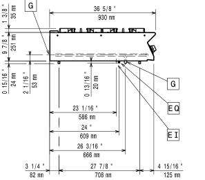
= Electrical inlet (power) EI G Gas connection
